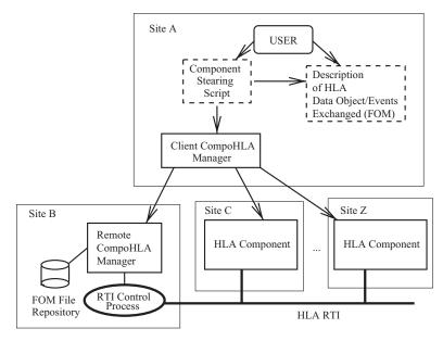
**Figure 6.4** Architecture of the CompoHLA environment. The user interacts with HLA components and the RTI control process via the Client CompoHLA Manager API accessible via a scripting language.
