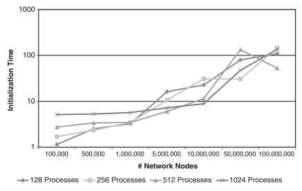
Figure 5.4 Initialization time by process count.
