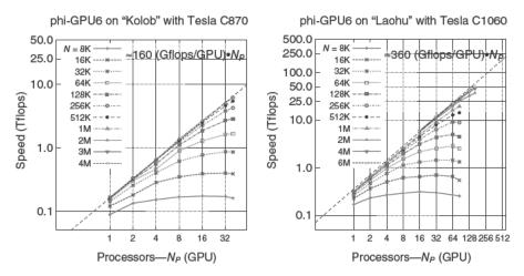
**Figure 3.3** Left: Same benchmark simulations as in Figure 3.2, but for the Frontier Kolob cluster with Tesla C870 GPUs at University of Heidelberg; 6.5 teraflops reached for 4 million particles on 40 GPUs. Right: NAOC GPU cluster in Beijing; speed in teraflops reached as a function of the number of processes, each process with one GPU; 51.2 teraflops sustained were reached with 164 GPUs (three nodes with 6 GPUs were down at the time of testing).
