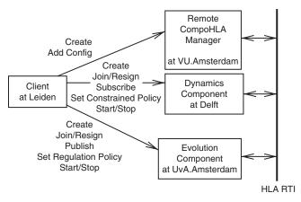
Figure 6.9 Setup of the HLA component experiment. Elements of the CompoHLA environment are installed on different sites on the DAS3 e-infrastructure and are called by the client script.
