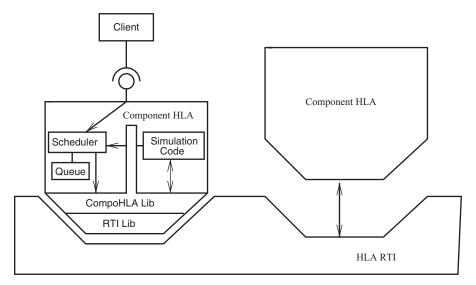
**Figure 6.6** Architecture of the HLA component plugged into the HLA RTI communication bus. The component exposes an interface for external requests. Thus, it is possible to change the state of the simulation in the HLA RTI layer by using an independent client.
