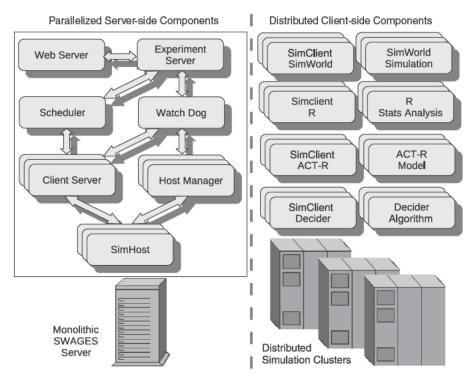
Figure 4.1 Overview of the SWAGES architecture in 2009 (all server-side components within the solid square on the left had to run on the same host computer).
