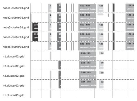
Figure 9.8 Example coallocations using advance reservation QosCosGrid capabilities for cross-cluster parallel simulations.
