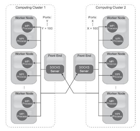
Figure 9.4 A new proxy technique for QCG-OMPI and QCG-ProActive based on SOCKS servers in QosCosGrid.
