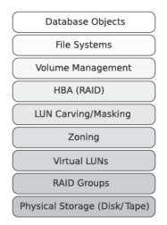
Figure 1.2 Simple storage model (Bunn et al., 2004). HBA, Host Bus Adapter; RAID, Redundant Array of Independent Disks; LUN, Logical Unit Number.
