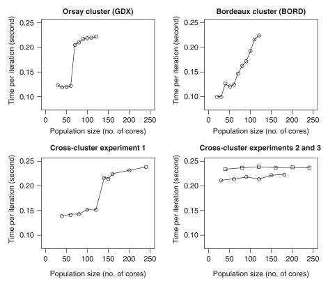
**Figure 8.4** Speedup results of the evolutionary algorithm using different clusters and computational resources. Note that the number of cores corresponds to the population size and hence the number of fitness calculations performed in an iteration. The graphs are discussed in the main text.
