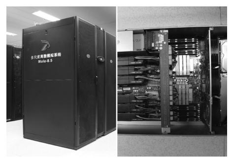
**Figure 3.4** Left: The Mole-8.5 Cluster at the Institute of Process Engineering in Beijing. It consists of 372 nodes, most with 6 Fermi Tesla C2050 GPUs. Right: single node of Mole-8.5 system (courtesy of IPE, photos by Xianfeng He).
