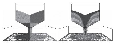
*Figure 2.1* Particle flow during hopper discharge. Particles are colored according to resultant force.
