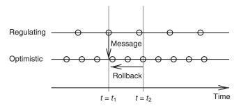
*Figure 6.2* Concurrent execution—optimistic approach. Both simulations can advance in time as far as needed, but a rollback becomes necessary if an outdated message is received.
