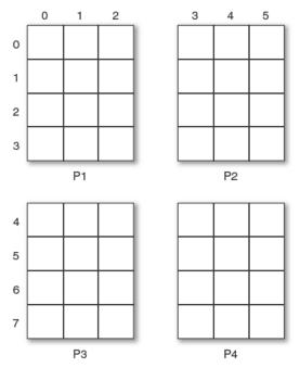
Figure 5.2 Distributed grid. P1 manages grid cells (0, 0)–(2, 3), P2 manages (3, 0)–(5, 3), and so on.
