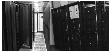
*Figure 3.1* Left: NAOC GPU cluster in Beijing, 85 nodes with 170 NVIDIA Tesla C1060 GPUs, 170-teraflop hardware peak speed, installed in 2010. Right: Frontier Kolob cluster at ZITI Mannheim, 40 nodes with 40 NVIDIA Tesla C870 GPU accelerators, 17-teraflop hardware peak speed, installed in 2008.
