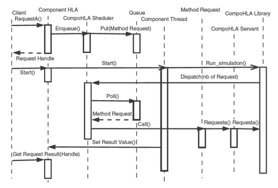
Figure 6.7 Time sequence diagram showing the interaction scenario between HLA component modules compliant with the active object pattern (Lavender and Schmidt, 1995). External requests are placed in a queue. Once the simulation starts, the scheduler is asked to dispatch the requests.
