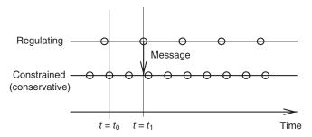
**Figure 6.1** Concurrent execution—conservative approach. The conservative constrained simulation can move forward as far as it is allowed by the regulating simulation.
