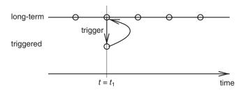
*Figure 6.3* Execution triggered by another simulation. One simulation launches the execution of another and waits for its results.
