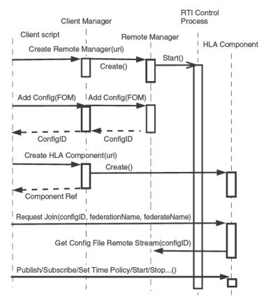
Figure 6.5 Time sequence diagram showing an interaction scenario within the CompoHLA environment when setting up a simulation from HLA components.
