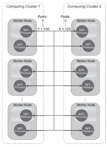
Figure 9.3 A typical port range technique used by administrators of computational resources for a cross-cluster communication.
