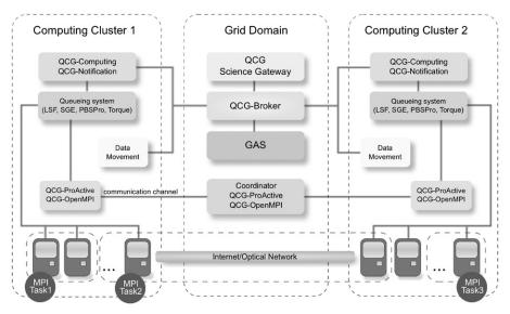
*Figure 9.5* The overall QosCosGrid architecture and its main services supporting QCG-OMPI and QCG-ProActive.
