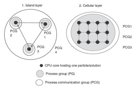
**Figure 8.3** Communication topology of the PSO algorithm. The arrows show the communication patterns in each process communication group: Communications in the island layer can be mapped onto a ring topology, while communications in the cellular layer can be mapped onto a spherical topology where each process communicates to its neighbors.
